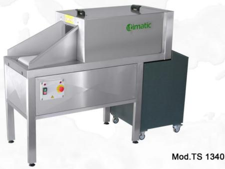
The Timatic HerbCut was designed and built in response to requests from cultivators and producers of delicate fresh and dried aromatic and medicinal herbs. But because of its innovative design and practical approach it can be used in cutting many other types of botanical material.
